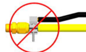
Figure 3: Unacceptable bond attachment on CSST
